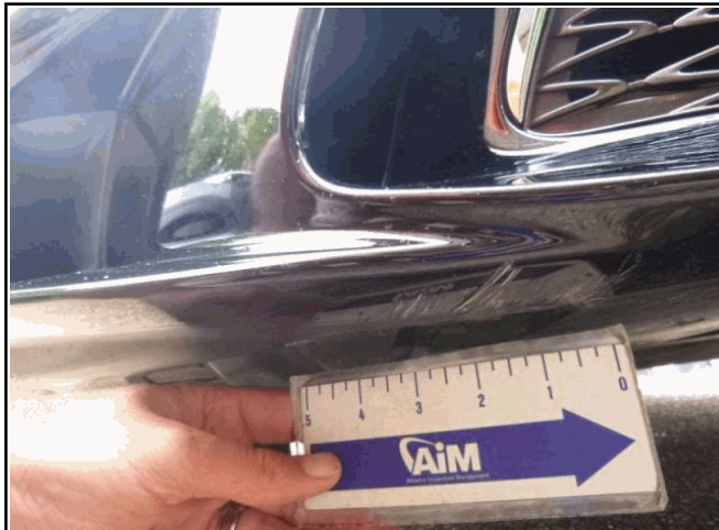
Picture Description : Bumper Cover Dented Bet 6" - 12"
